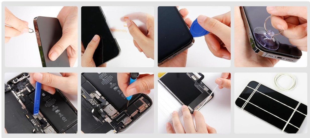
Image 2.2: A comprehensive set of tools provided for the screen replacement, including screwdrivers, prying tools, suction cup, SIM ejector, and adhesive strips.
