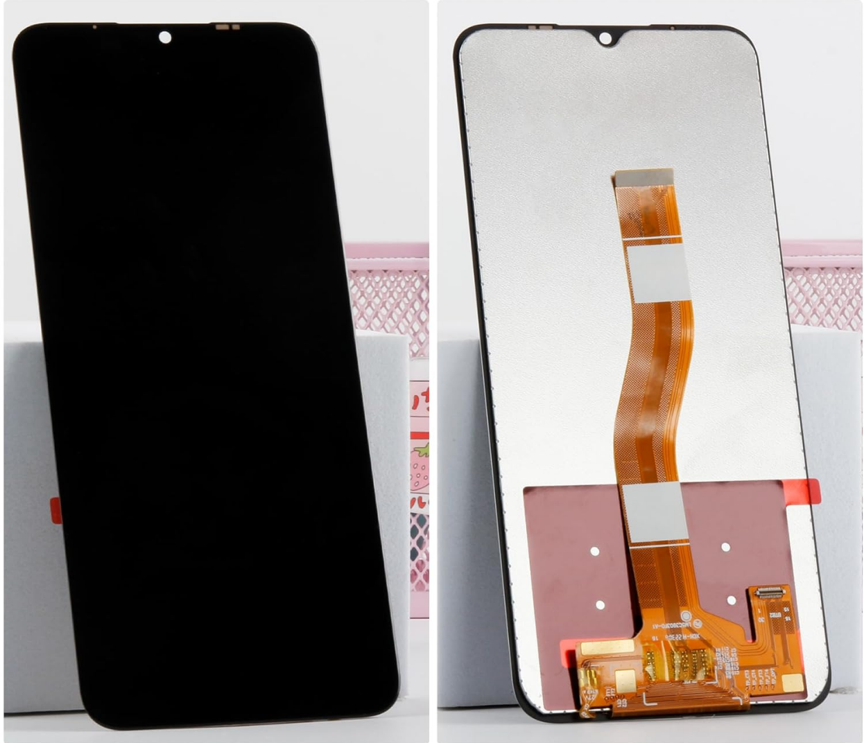
Image 2.1: Front and back views of the LCD display assembly without the phone frame, showing the display surface and the flex cable connections.
