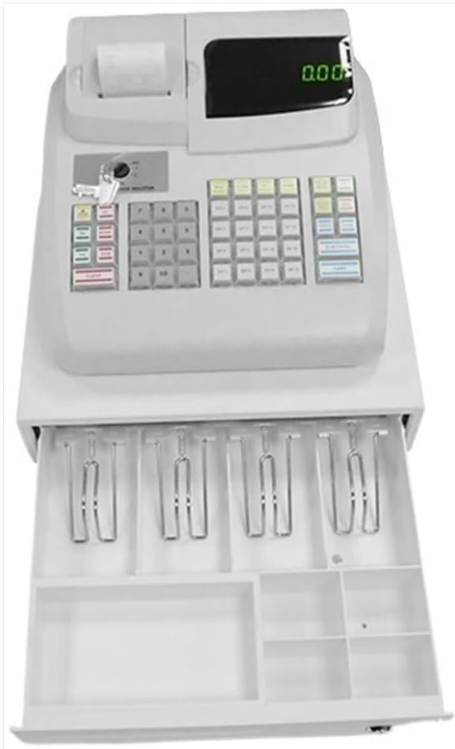
Figure 2: Front view of the cash register, showing the receipt printer and cash drawer.
