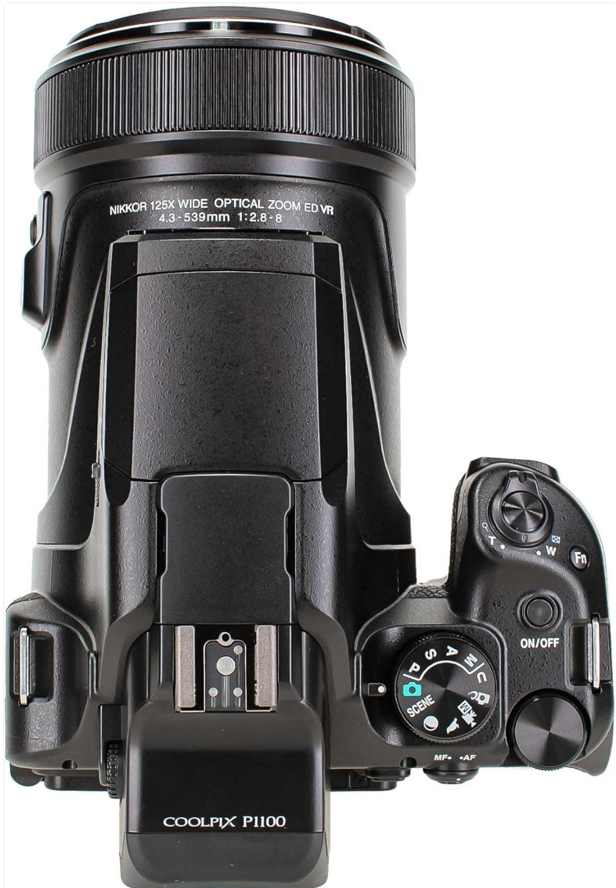
Figure 4.1.1: Top view of the Nikon COOLPIX P1100, highlighting the mode dial and the ON/OFF button.
