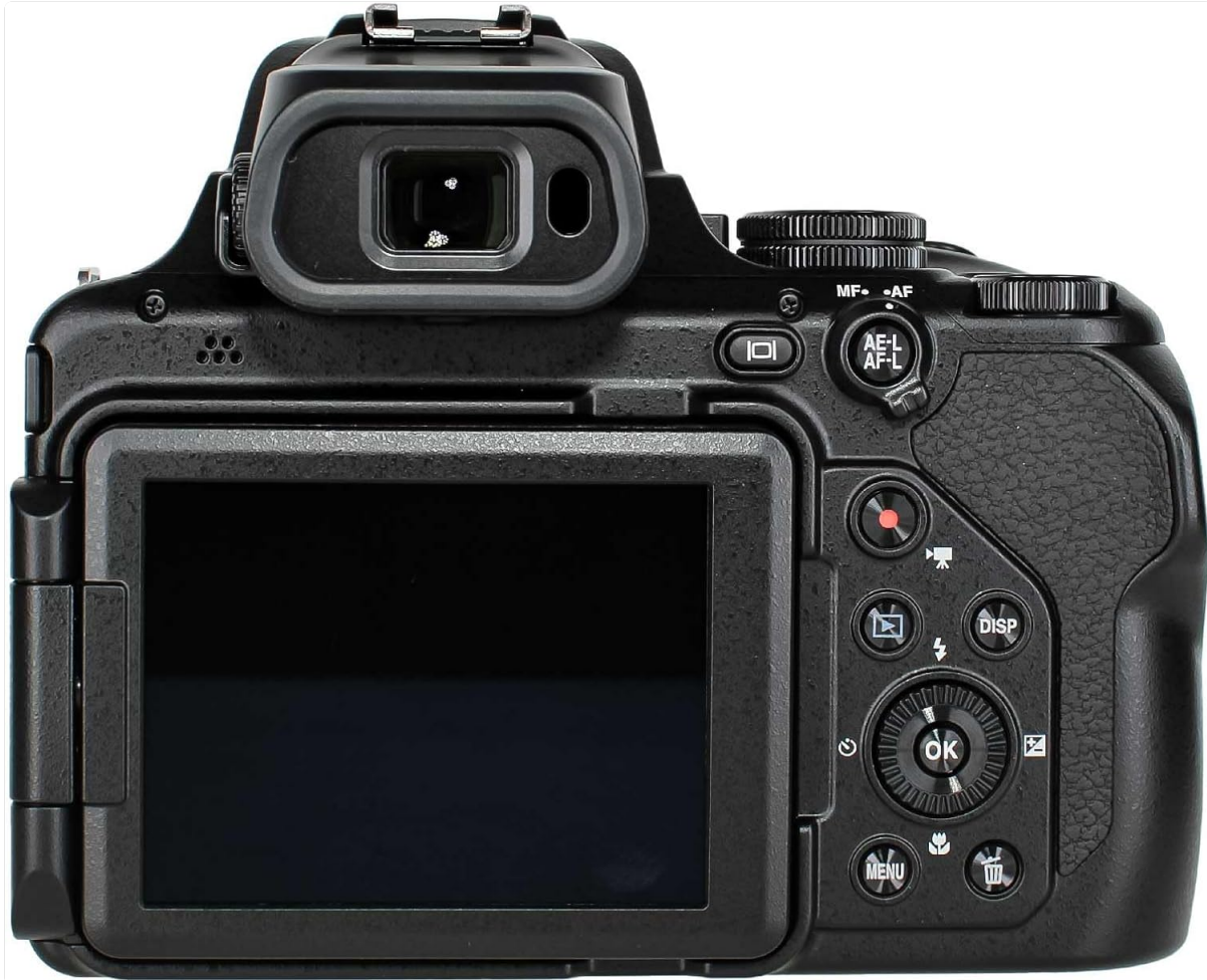
Figure 4.2.1: Rear view of the Nikon COOLPIX P1100, displaying the vari-angle LCD screen and various control buttons for navigation and settings.
