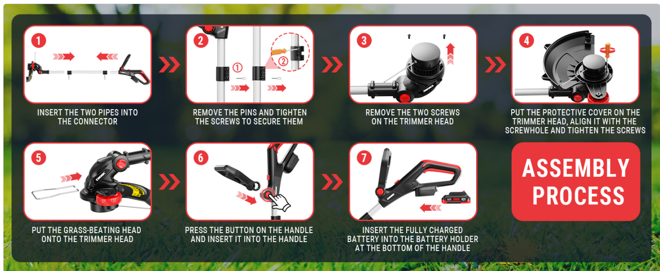
Figure 3.1: Visual guide for the assembly process of the string trimmer.
