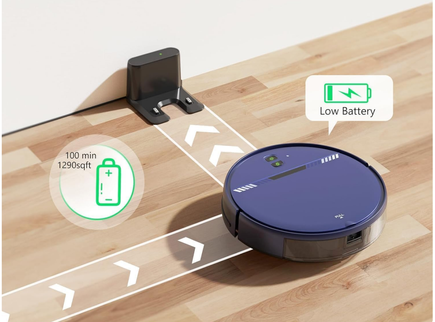
Figure 3: The robot vacuum automatically returning to its charging dock when the battery is low, illustrating its self-charging capability.
