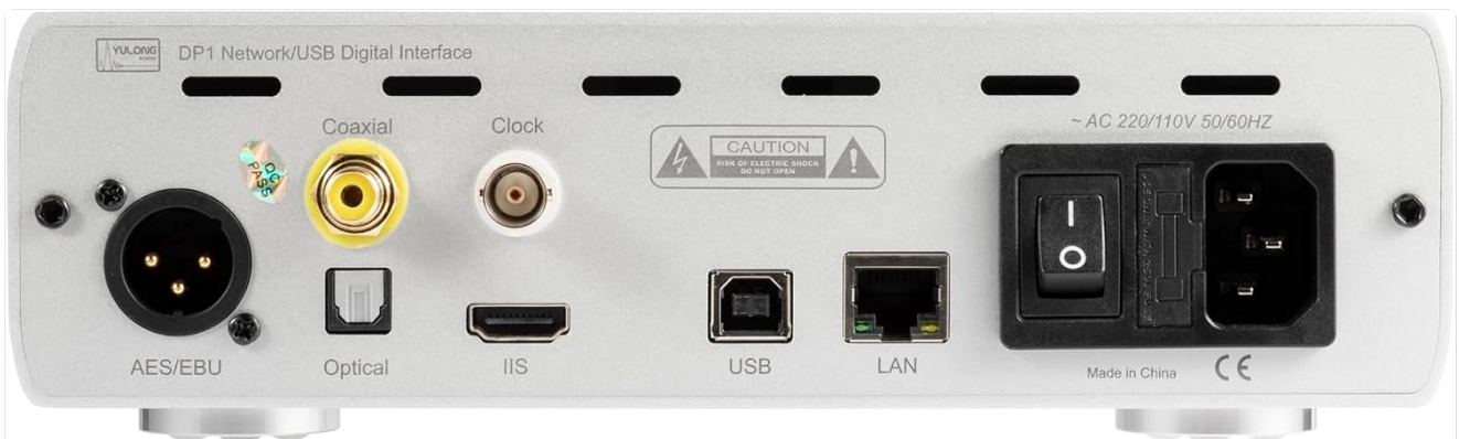
Figure 3.2: Rear view of the YULONG DP1, illustrating the various input and output ports including AES/EBU, Optical, Coaxial, IIS, USB, LAN, Clock input/output, and AC power input.
