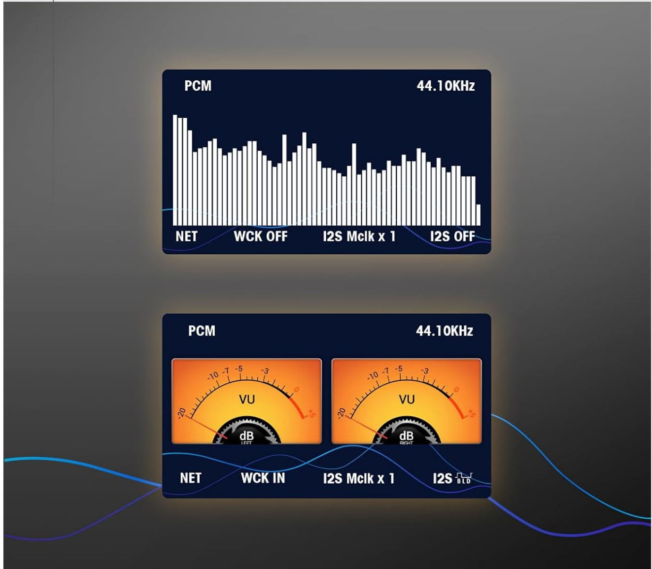
Figure 5.1: Examples of the DP1's IPS LCD screen displaying different visual modes, such as a real-time spectrum analyzer and classic analog-style VU meters, providing visual feedback on the audio signal.
