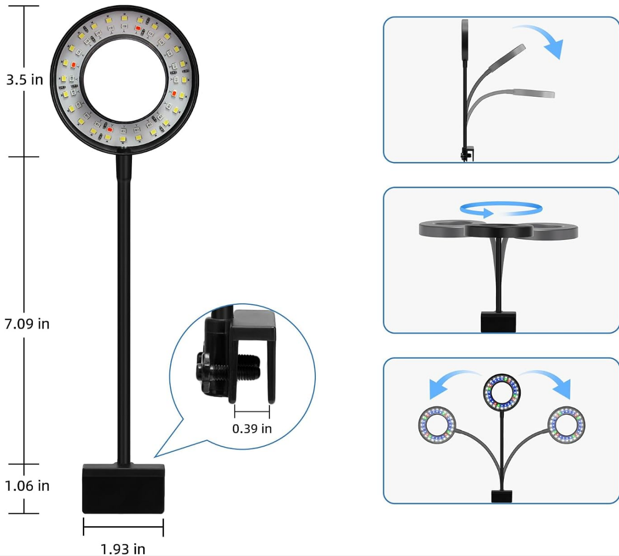
Figure 5: 360° Rotating Gooseneck Design. The diagram illustrates the adjustable gooseneck, allowing for flexible positioning and optimal light direction.
