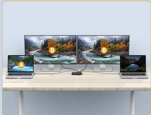
Image 5.2: Examples of display configurations for Windows (MST mode) and macOS (SST mode) when using the KVM switch with dual monitors.
