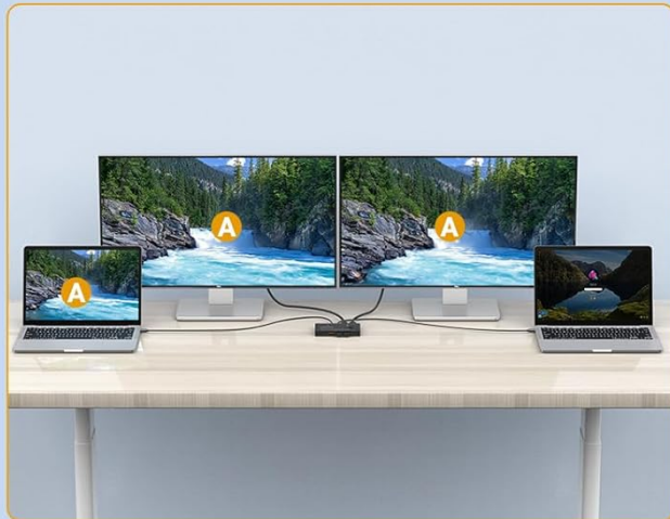
Image 5.2: Examples of display configurations for Windows (MST mode) and macOS (SST mode) when using the KVM switch with dual monitors.
