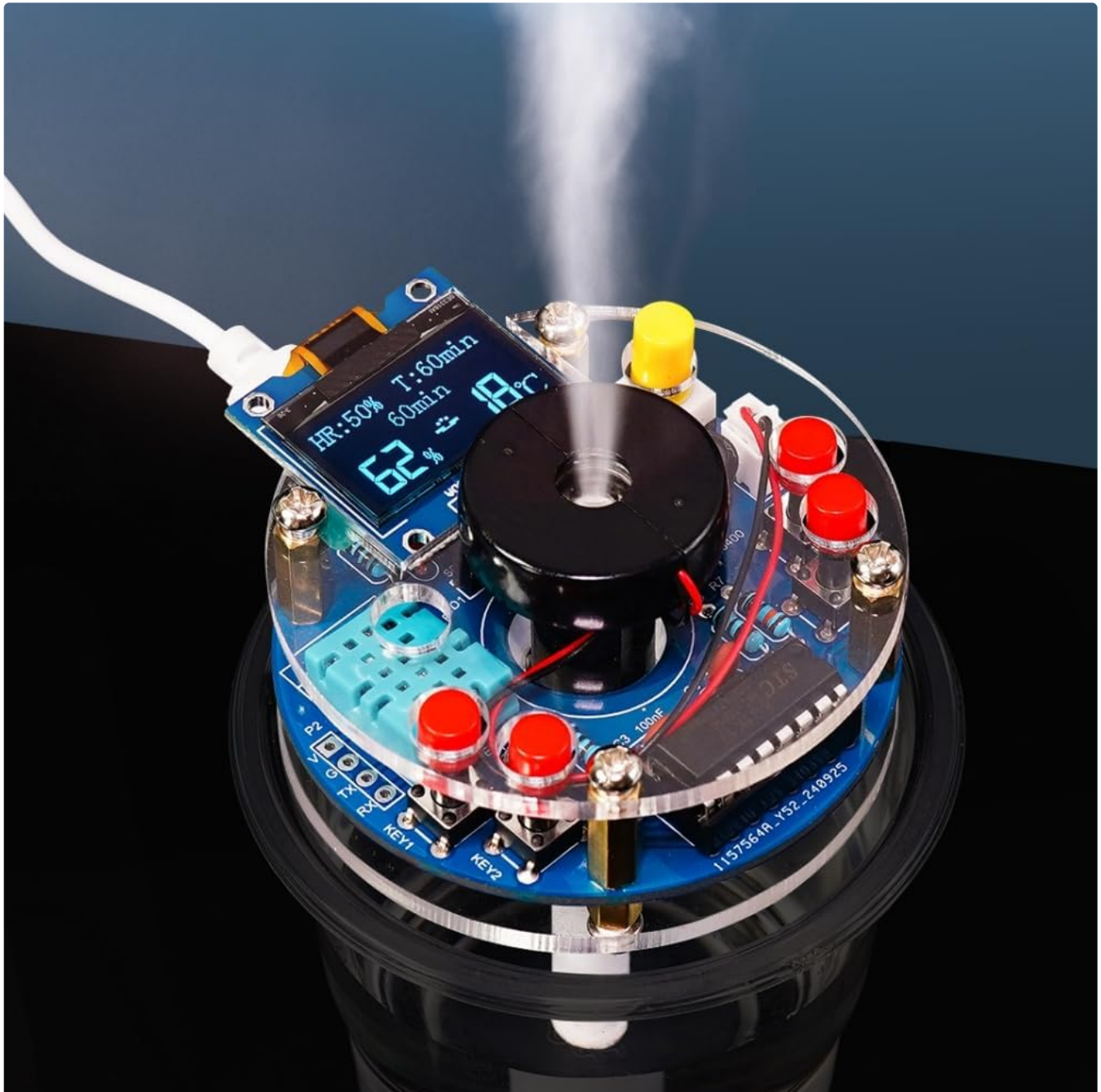
Image: The humidifier actively producing mist, with the OLED screen displaying operational data.
