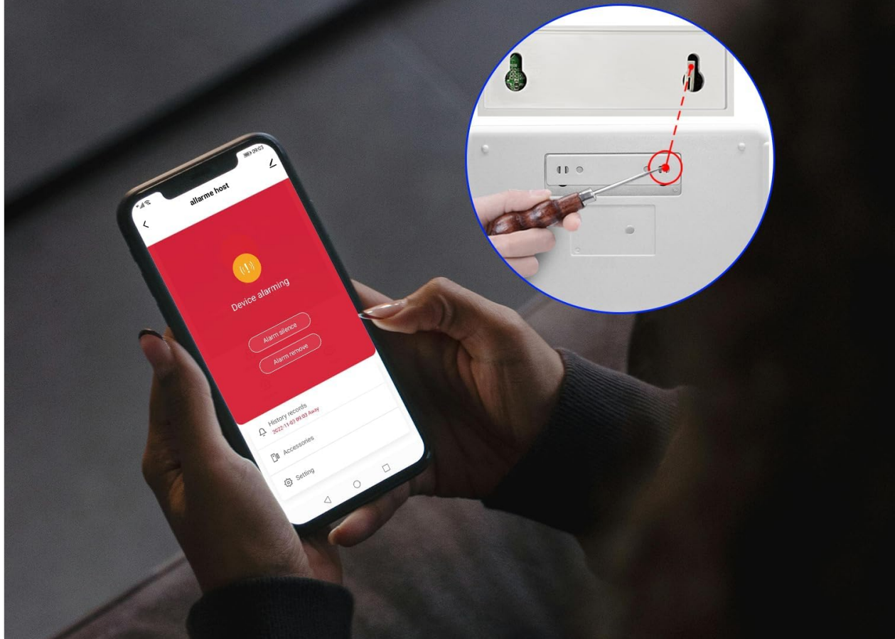
Figure 5.2: The anti-demolition alarm function, where removing the device triggers an alert on the host and sends a notification to the user's phone.
