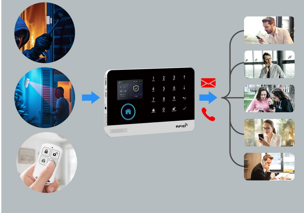
Figure 4.2: The system supports 5 preset alarm calls, ensuring no alarm information is missed. If a busy line is encountered, it will dial the next reserved number.
