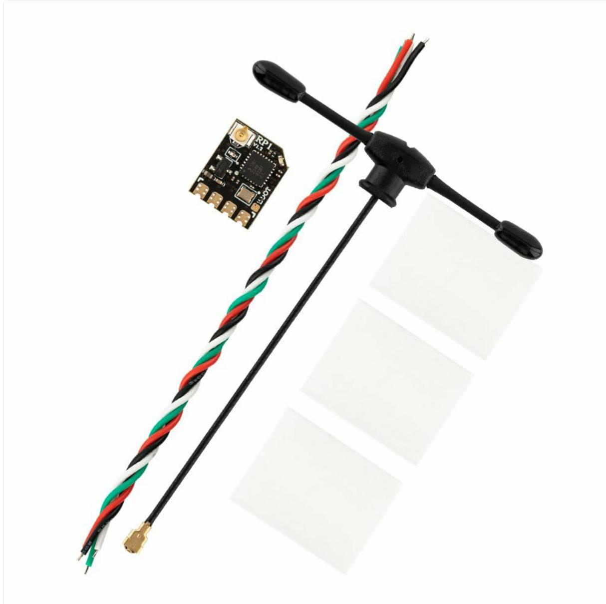
This image displays the RadioMaster RP1 V2 Nano ExpressLRS Receiver, highlighting its compact dimensions of 13mm in length, 11mm in width, and 3mm in height. The image shows the UFL antenna connector and solder pads.
