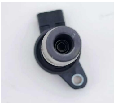
Figure 5: Top view of the ignition coil, showing the internal contact for the spark plug.
