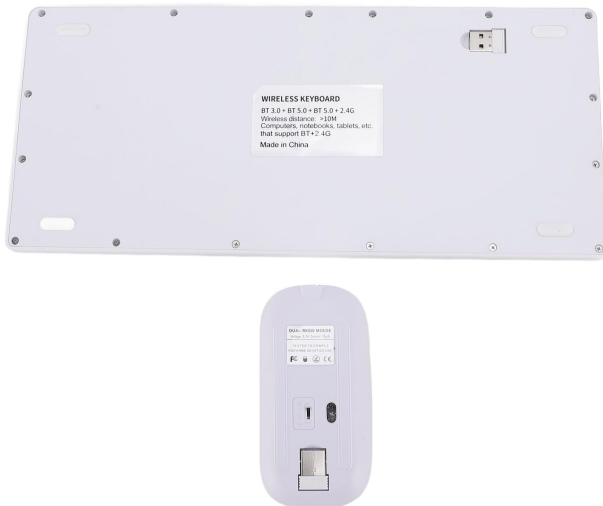
Rear view of the keyboard and mouse. The keyboard displays its wireless specifications. The mouse shows its power switch and the compartment for the shared USB receiver.
