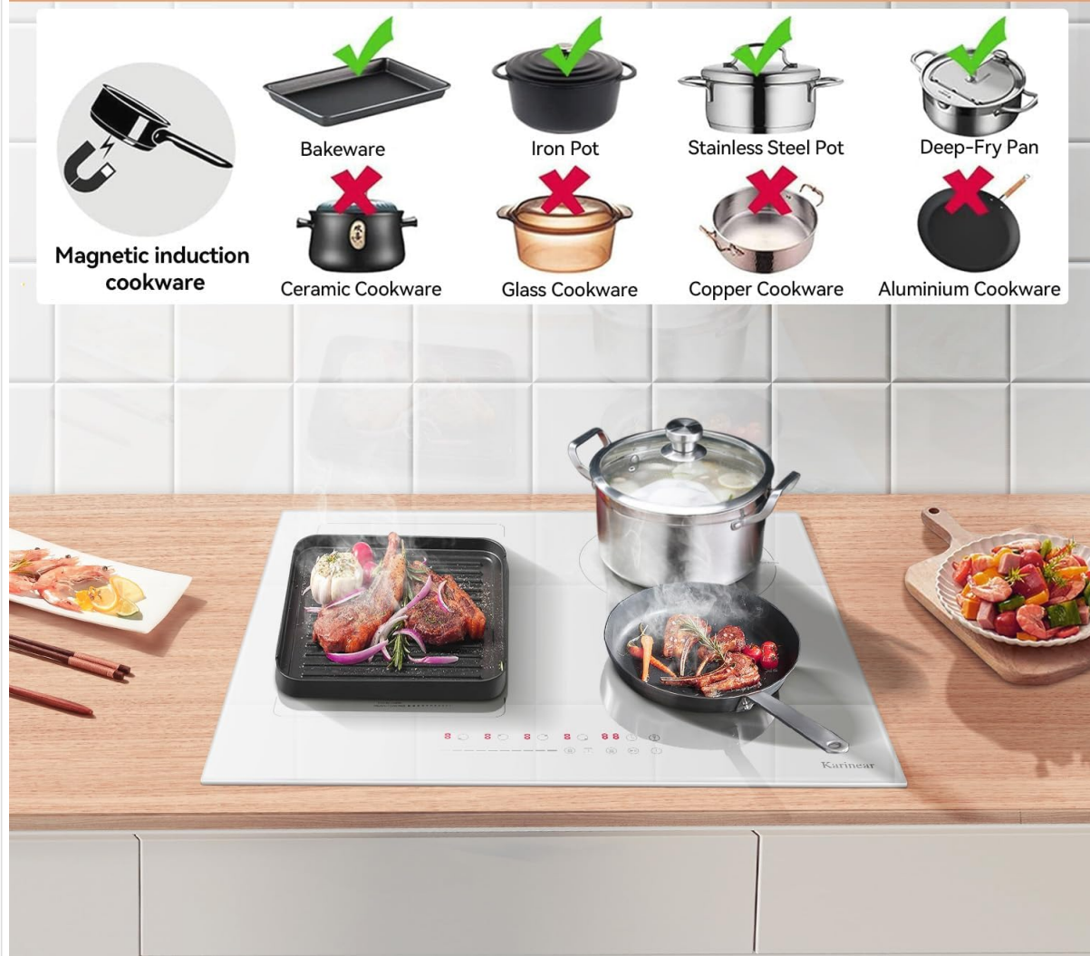
Figure 5.4: Cookware Compatibility. This image illustrates which types of cookware work with induction cooktops (e.g., cast iron, stainless steel with magnetic base) and which do not (e.g., ceramic, glass, copper, aluminum without magnetic base).
