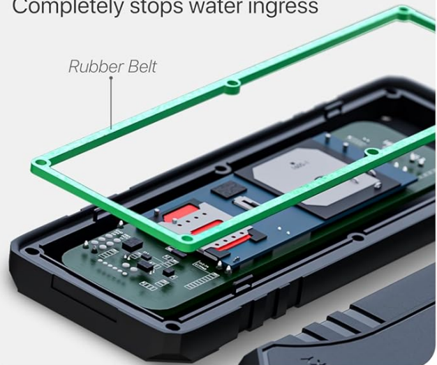
Figure 7.1: Waterproofing features and internal shield protection.
