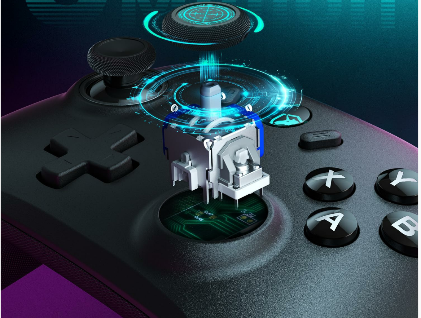
Figure 4: Internal mechanism of the Hall Effect Joysticks, highlighting their durable and precise design for extended use.
