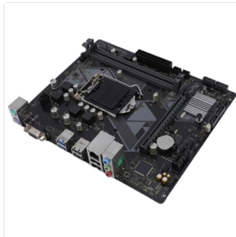
Image: Close-up of the motherboard's two DDR4 DIMM slots and multiple SATA III ports for memory and storage expansion.
