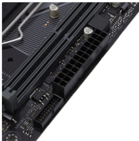
Image: A view of the motherboard highlighting the solid capacitors and 8-pin and 24-pin power connectors for stable power delivery.
