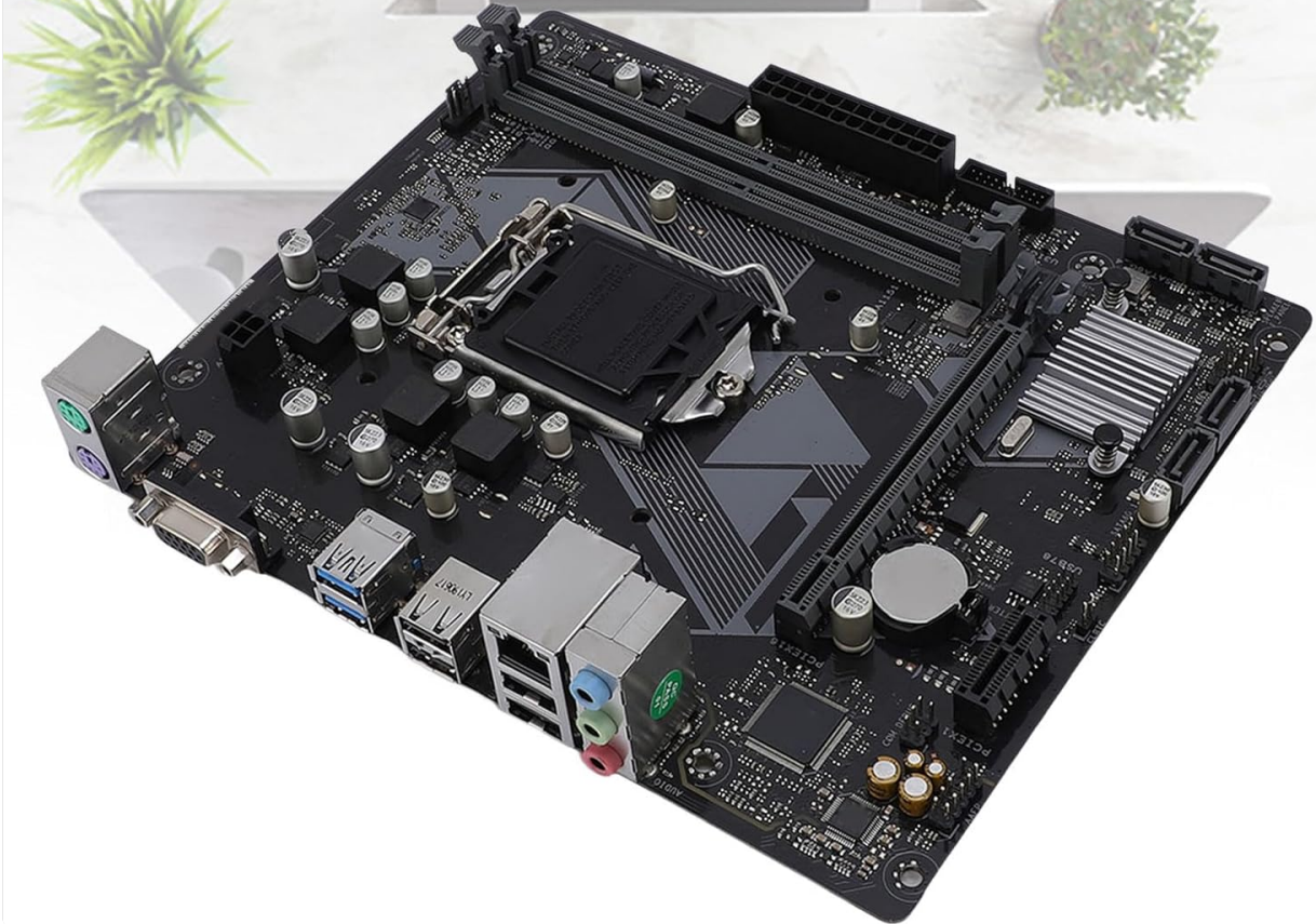
Image: Angled view of the motherboard, highlighting the two DDR4 DIMM slots.
