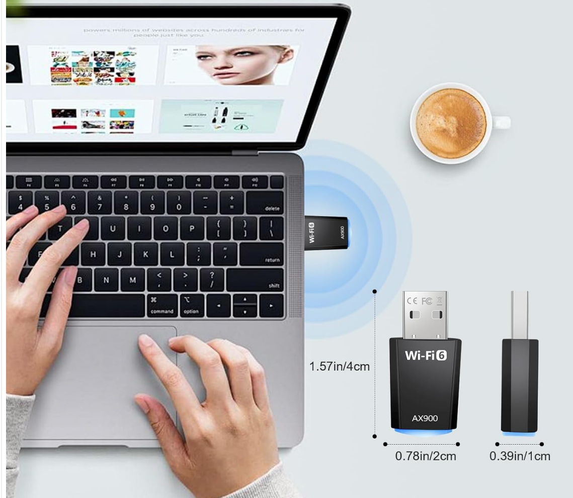
Figure 2.5: The Vemfay AX900 adapter plugged into a laptop, demonstrating its compact size and portability. Dimensions are shown as 1.57 inches (4cm) length, 0.78 inches (2cm) width, and 0.39 inches (1cm) thickness.
