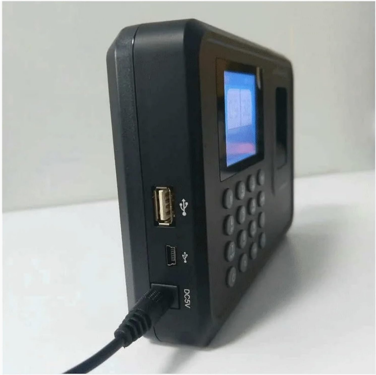
Image 3.1: Side view of the EliteBloom X1, showing the USB port and DC5V power input.
