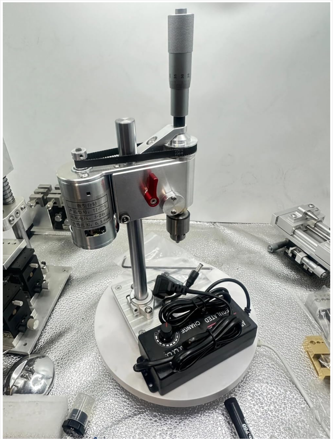
Figure 3: Detail of the motor housing and the power adapter with speed control.
