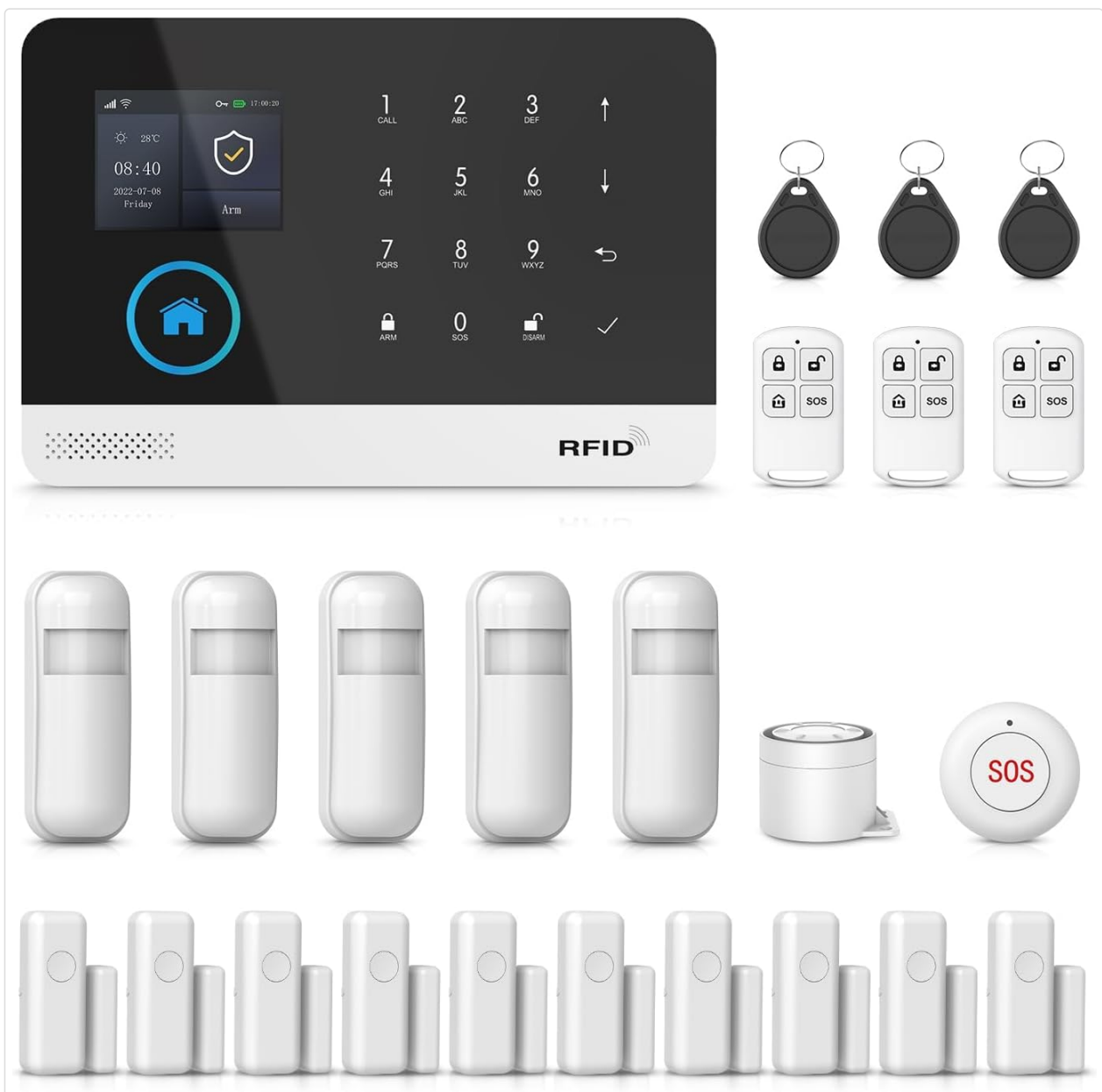
Image: Overview of the PGST Wireless WiFi Home Alarm System, showing the main panel, motion sensors, door/window sensors, remote controls, and RFID tags.
