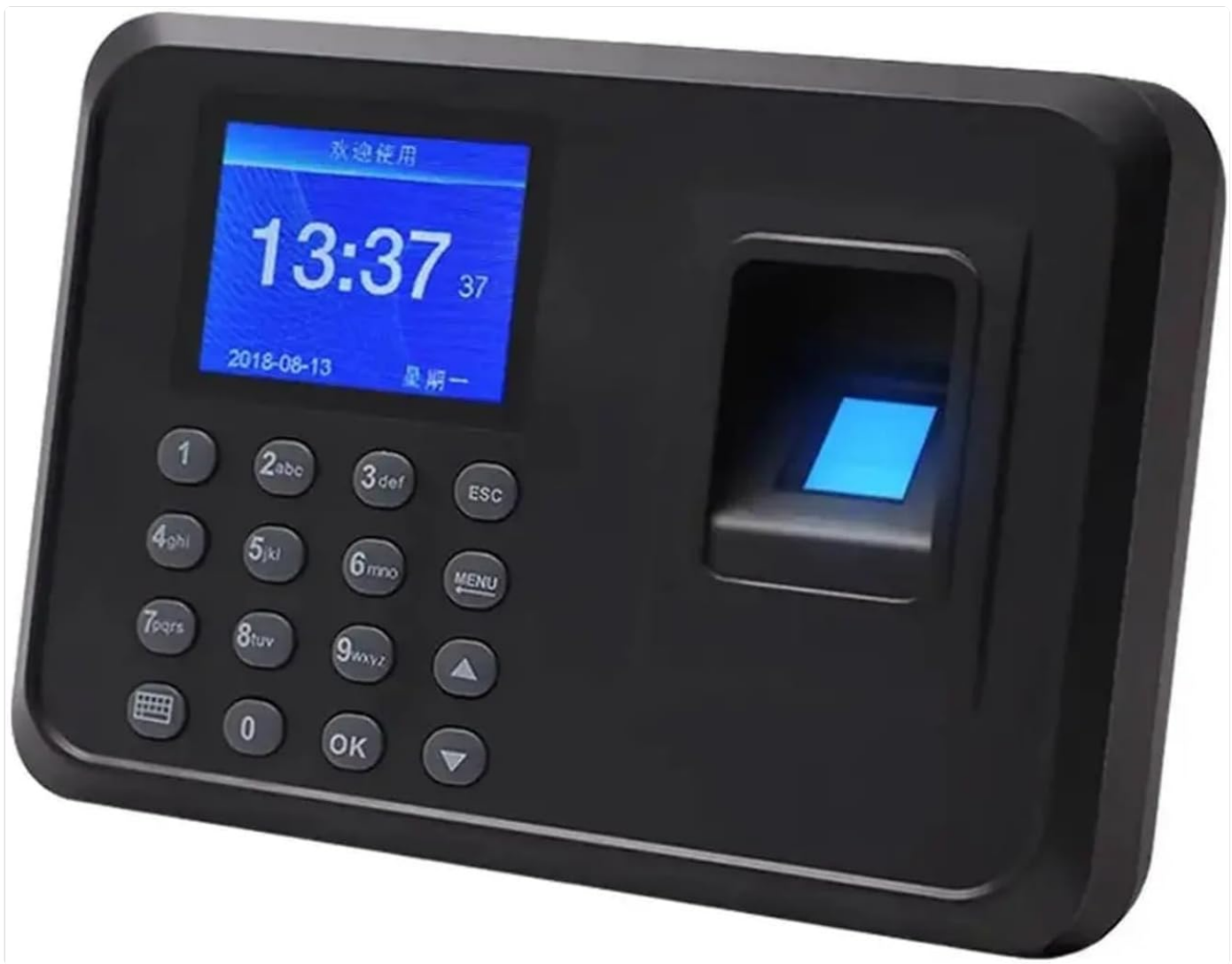
Figure 1: Front view of the UMJIGF F01 Fingerprint Attendance Machine, showing the screen, keypad, and fingerprint scanner.
