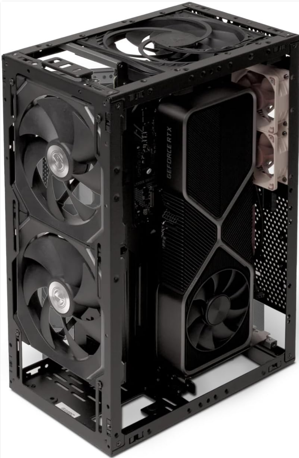
Figure 4.1: Internal view showing a graphics card and cooling fans installed, highlighting internal layout.
