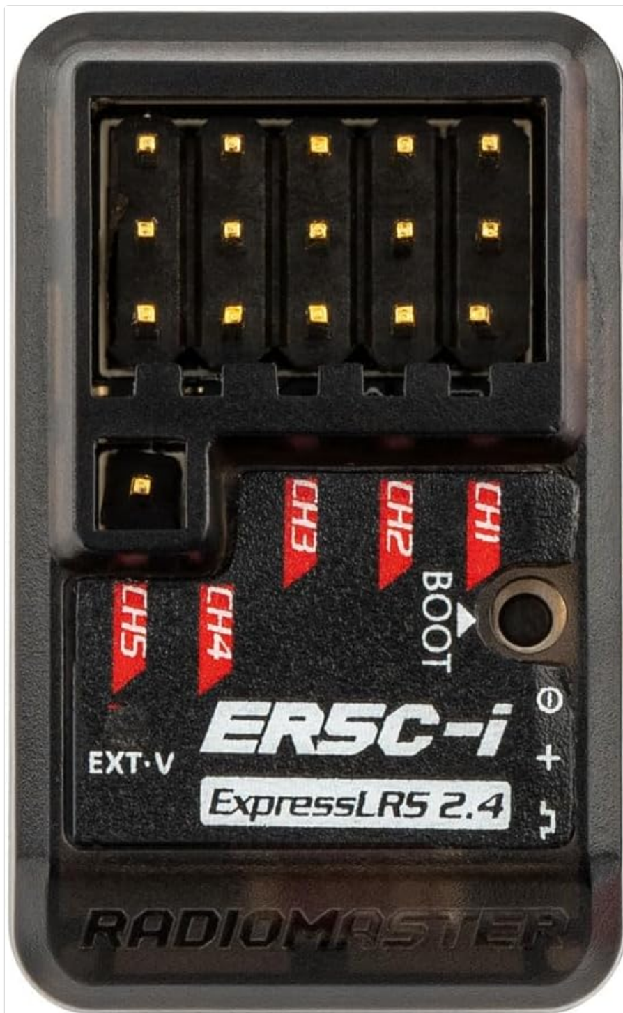
Image: Top view of the ER5C-i receiver, highlighting the five PWM output channels (CH1-CH5), the boot button, and the EXT-V port.
