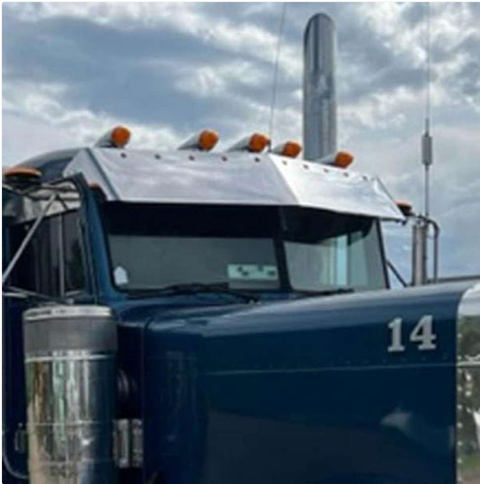
Figure 1: The Technical Precision 14-inch Stainless Steel Blind Mount Drop Visor with 10 Bullseye LED Lights, shown installed on the front of a Peterbilt 388 truck. The visor is positioned above the windshield, featuring multiple amber LED lights along its edge, enhancing visibility and the truck's aesthetic.
