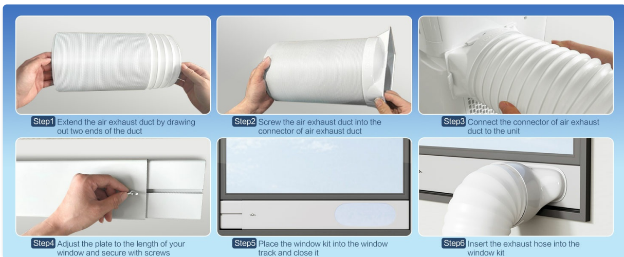
Figure 7: Detailed steps for exhaust hose and window kit assembly.
