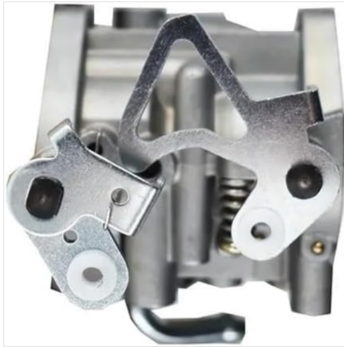
Figure 5.1: Top view of the carburetor, showing the throttle and choke linkage mechanisms.
