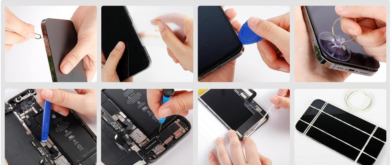
Image: A visual sequence illustrating the typical steps involved in replacing a smartphone screen, from opening the device to installing the new display, emphasizing the use of specialized tools.
