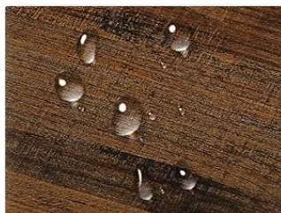
Image 5.1: The water-resistant surface of the desk, showing how liquids bead on the finish.
