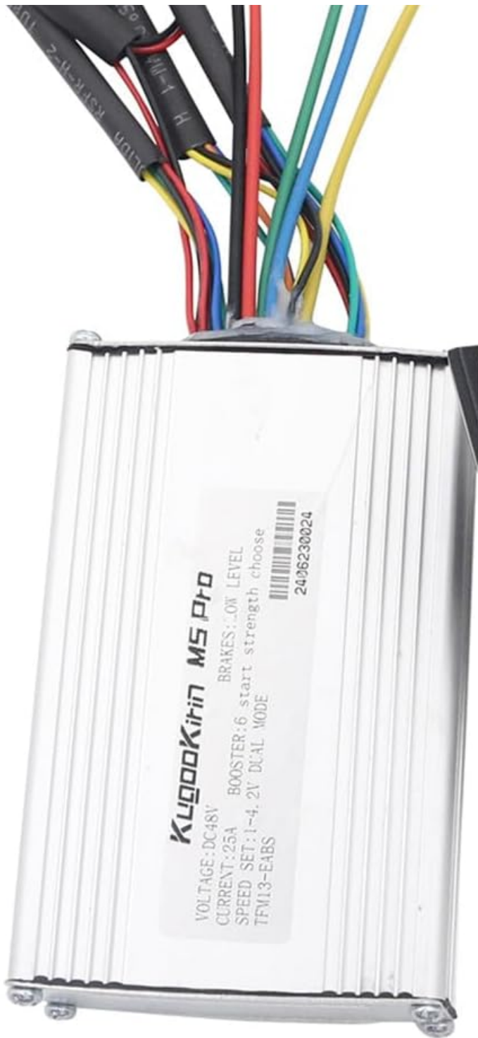
Image 2: A detailed view of the SPEDWHEEL controller, highlighting the product label with voltage and current specifications, and the organized arrangement of its various output wires.
