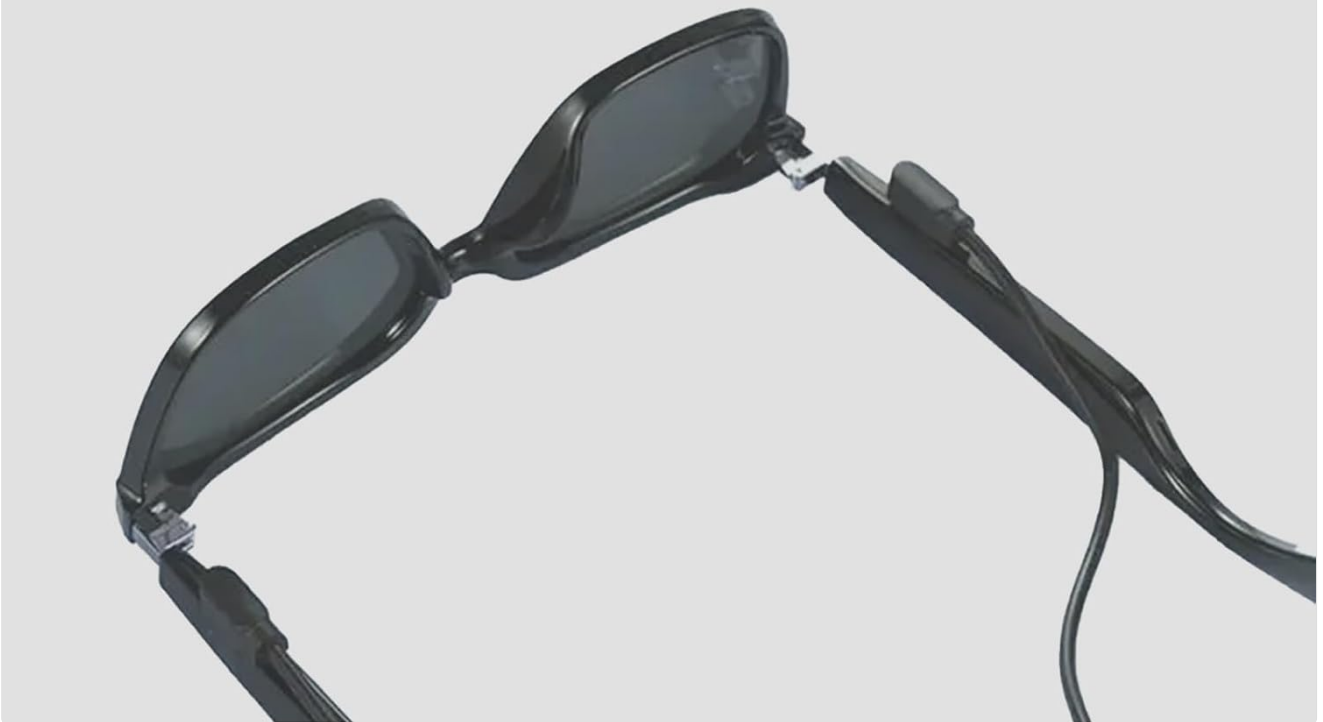
Figure 3: The cable allows for simultaneous charging of both sides of the smart glasses.
