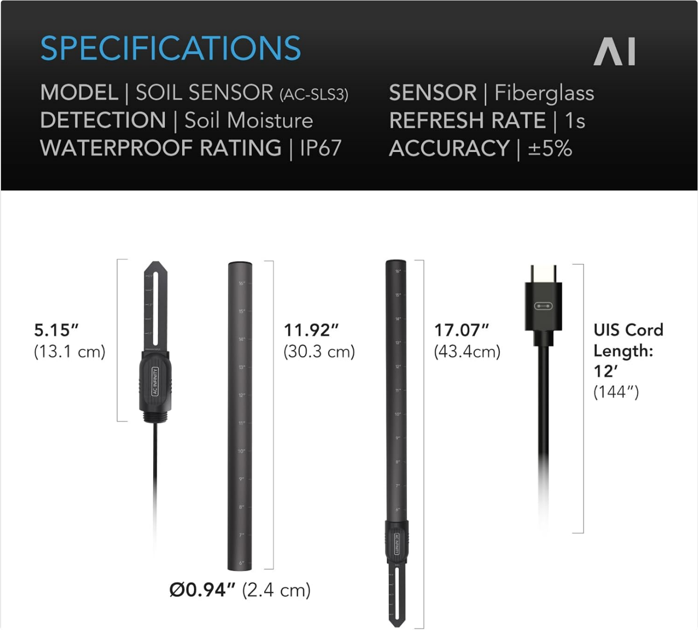
Figure 5: Detailed dimensions and specifications of the AC Infinity Soil Sensor Probe.
