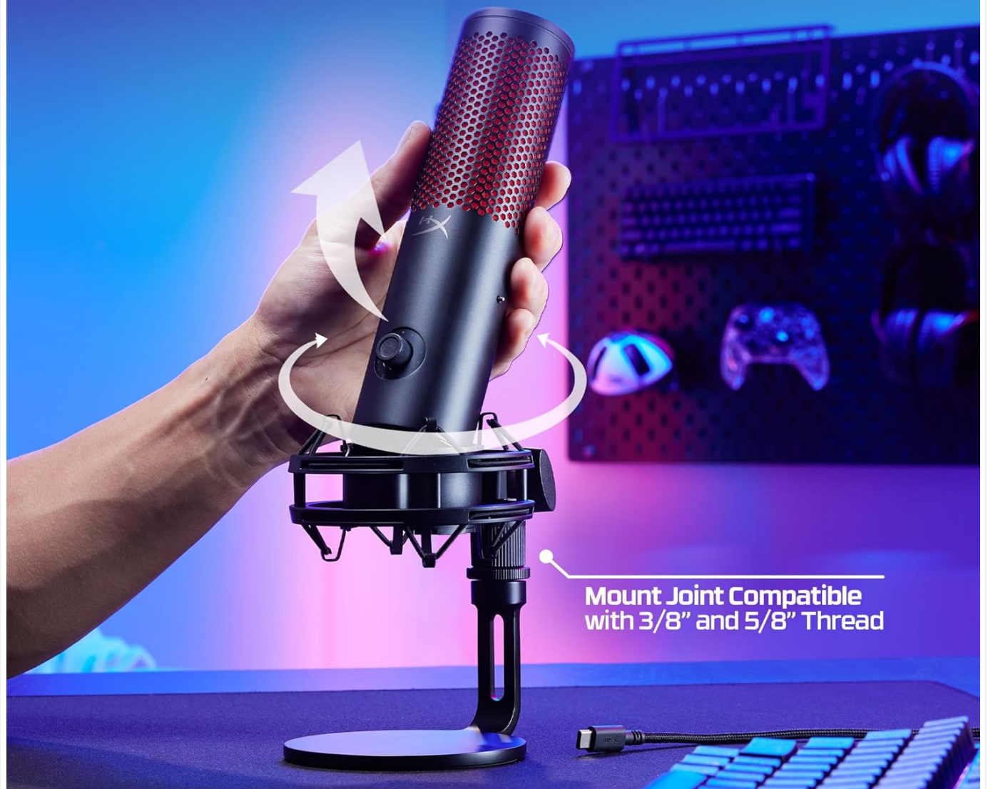
Figure 1: Removable Shock Mount. The microphone can be easily detached and reattached from its integrated shock mount, which helps to reduce vibrations and handling noise.
