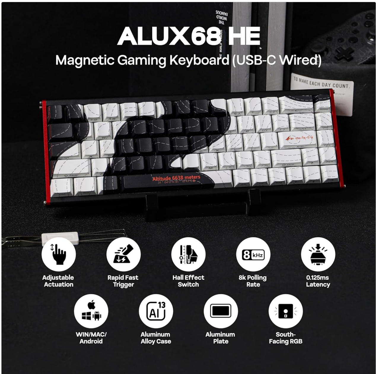
Image 4.1: Visual summary of the keyboard's main features, including adjustable actuation, rapid trigger, Hall Effect switches, and 8K polling rate.
