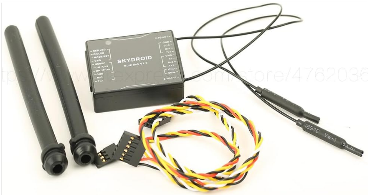
Figure 2.1: Overview of the Skydroid T12/SG12-RX Receiver and its accompanying accessories, including the main
