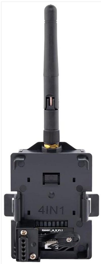
Rear view of the module, showing the connection points and the JR adapter.
