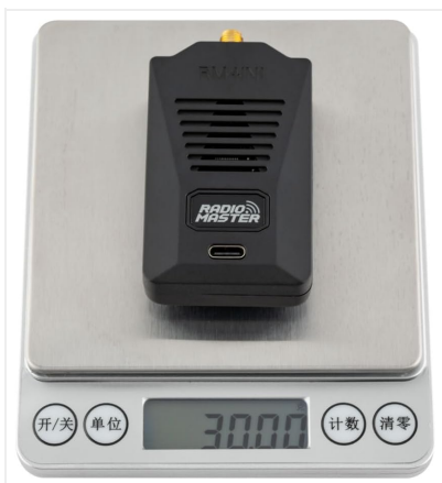
The module's weight is approximately 30 grams, as shown on a digital scale.
