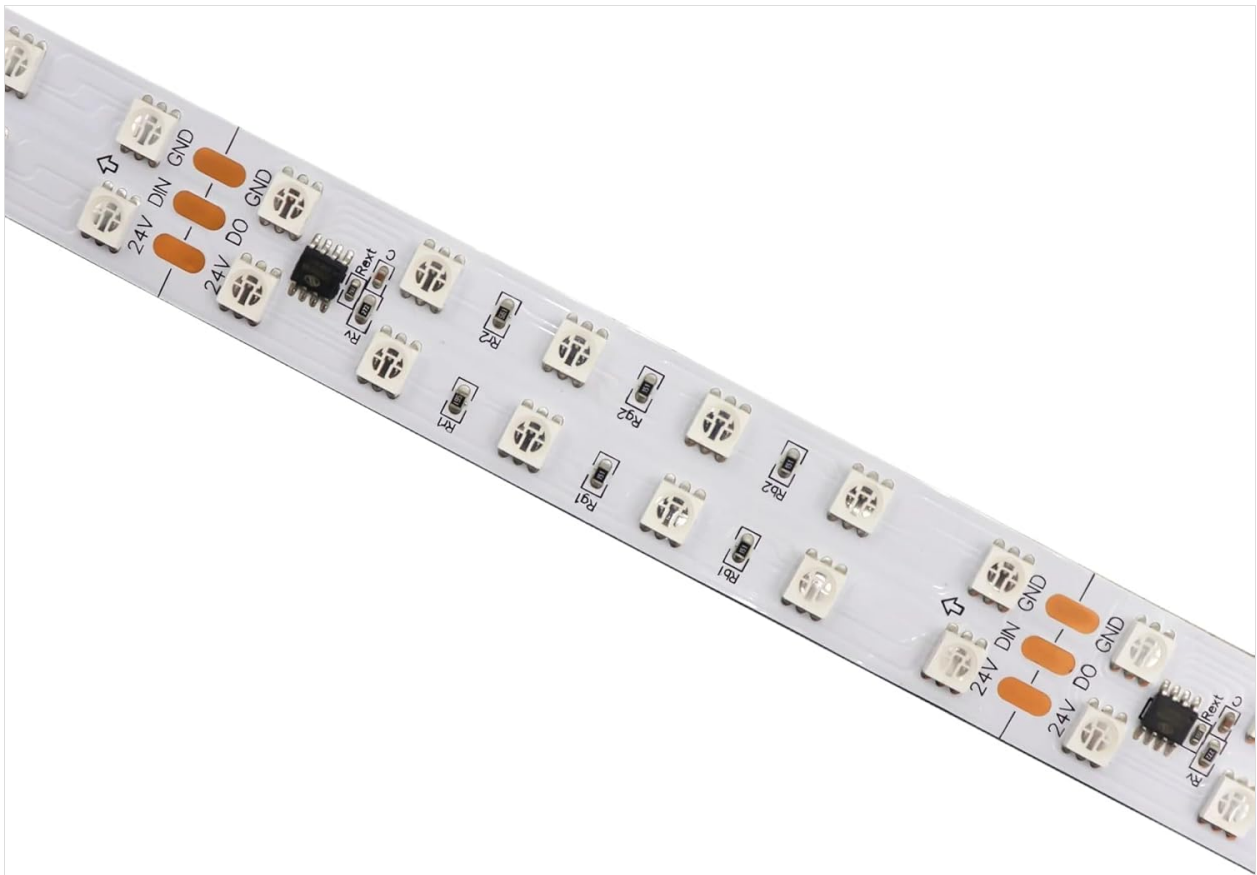
Image: Detail of the 24V LED strip, showing similar components to the 12V version but with '24V' markings for power input.
