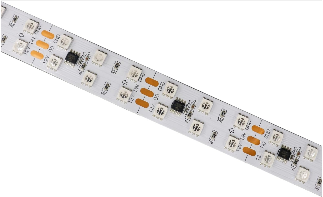
Image: Detail of the 12V LED strip, highlighting the 5050 SMD RGB LEDs and the integrated control ICs, along with connection points for power and data.
