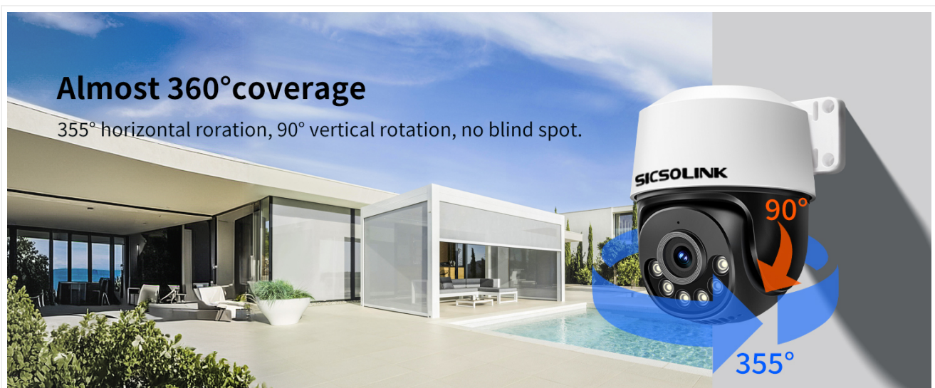
Figure 5: 355° Pan and 90° Tilt Coverage
