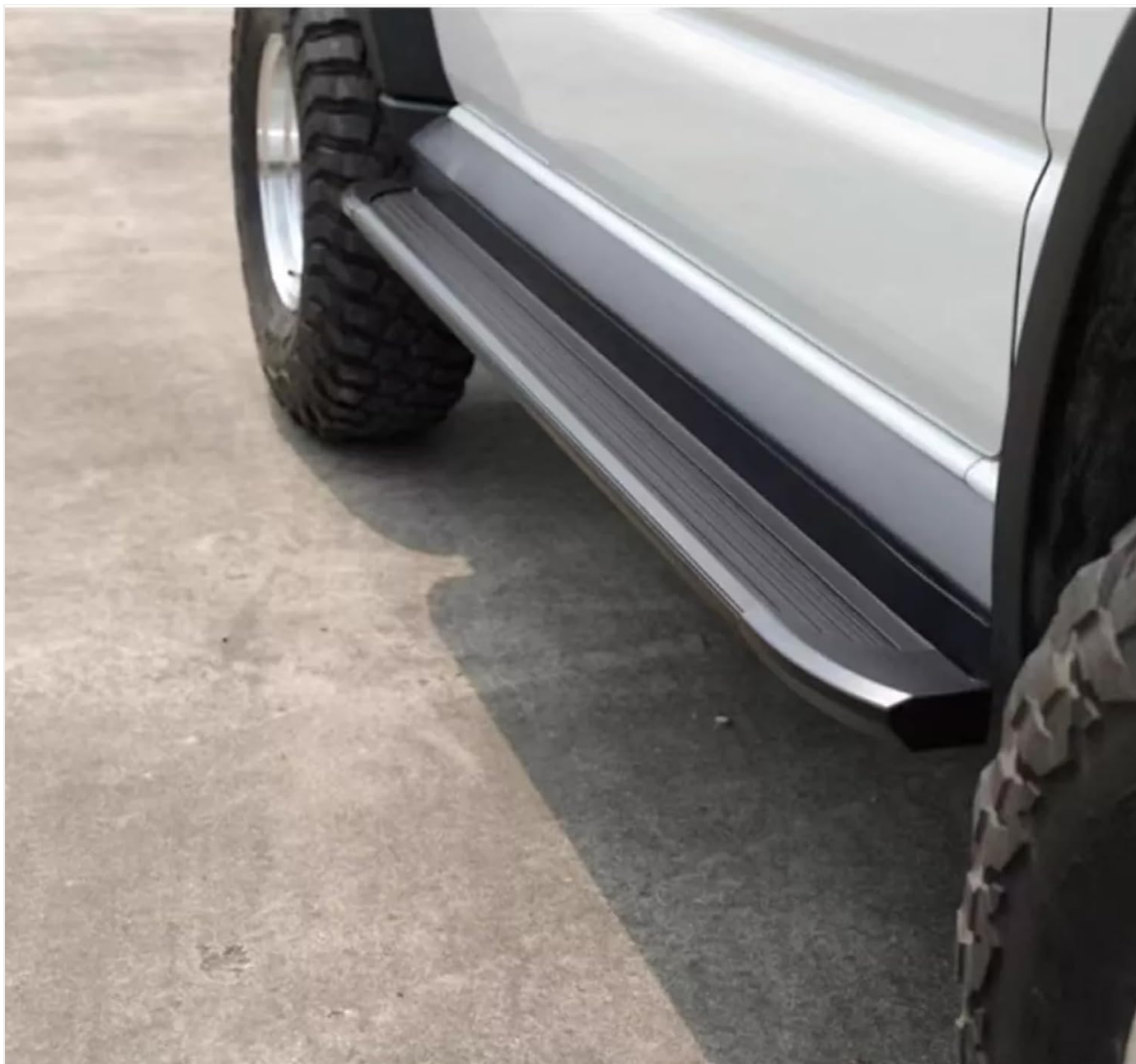
Image: A close-up view of the running board successfully installed on the side of a Suzuki Jimny, demonstrating its flush fit and appearance.
