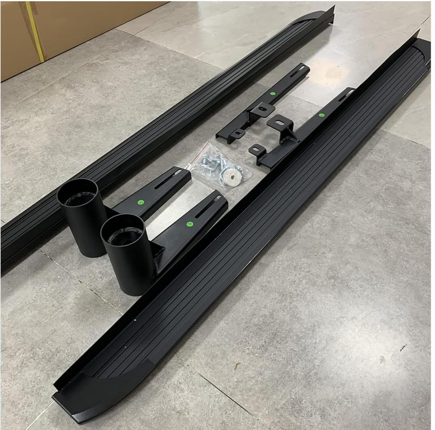
Image: Overview of the running board components, showing the two main boards, various mounting brackets, and a bag of installation hardware.
