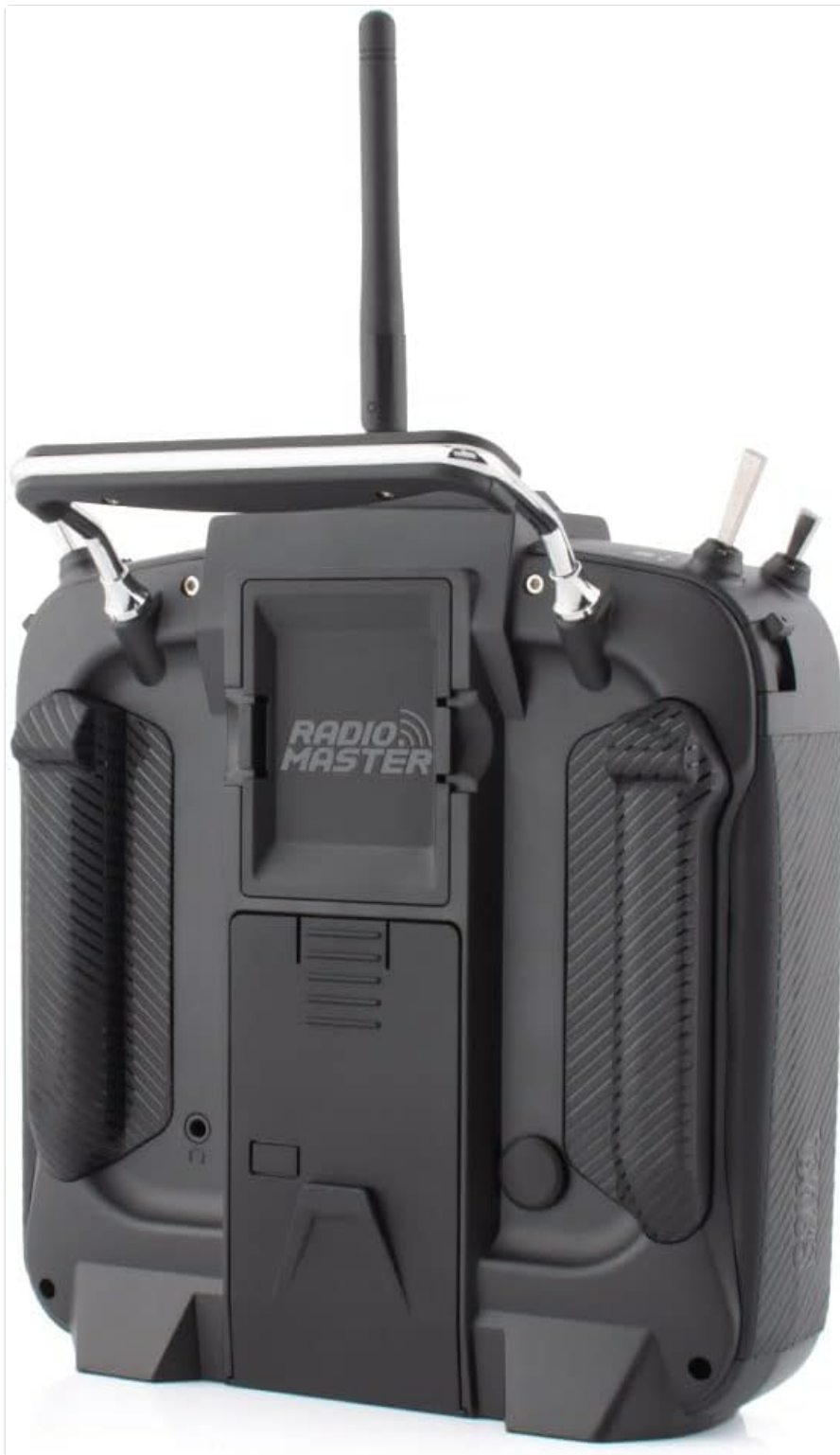
Figure 3: Rear view of the RadioMaster TX16S MKII V4.0 transmitter, showing the battery compartment and handle.
