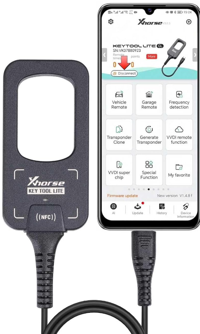
Figure 3: The Key Tool Lite connected to an Android phone, displaying the application interface.
