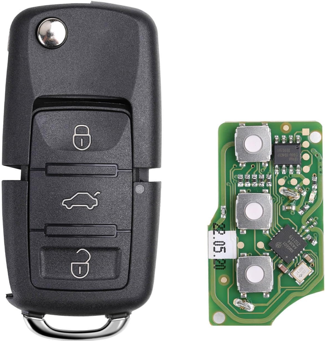
Figure 6: A typical key remote disassembled, showing the external casing and the internal circuit board.
