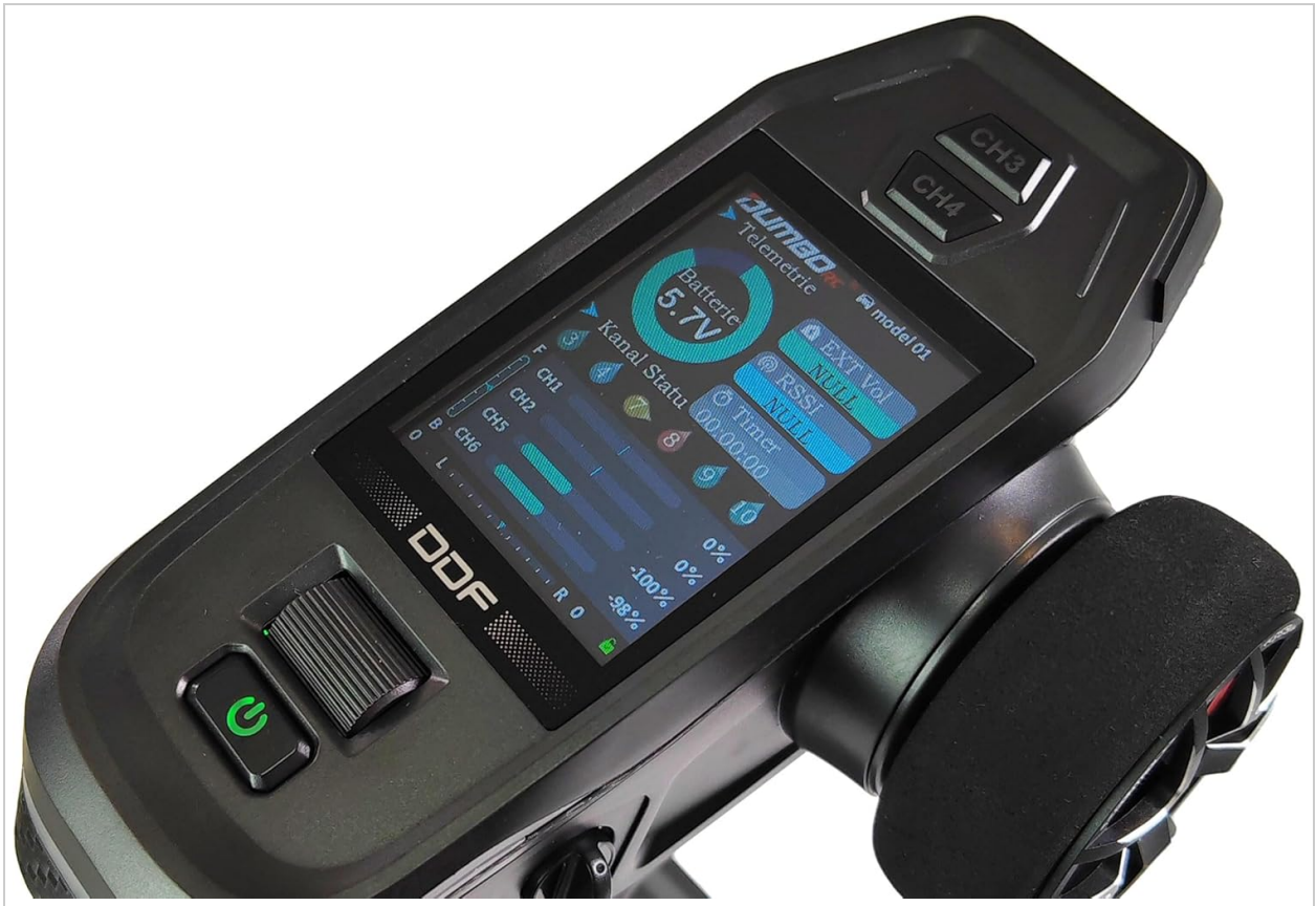
Figure 3.3: The DDF-350's color display, showing real-time telemetry data such as battery voltage, RSSI, and channel status. The menu allows for extensive programming.
