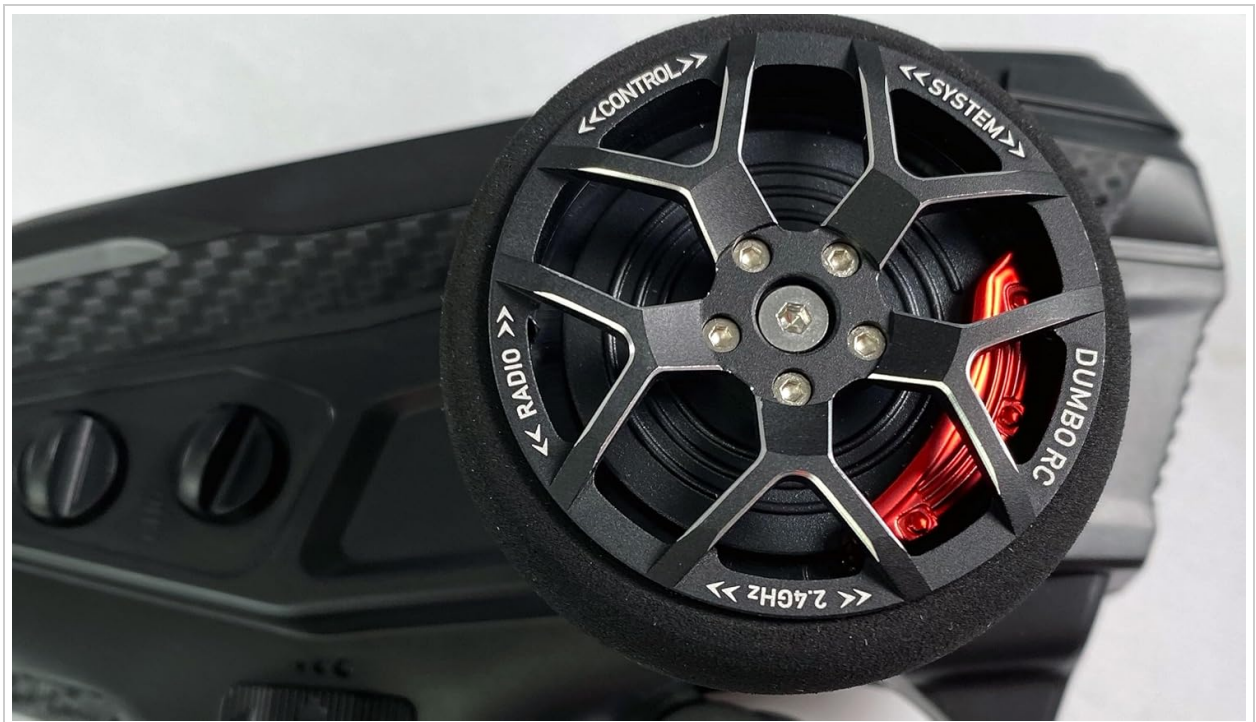
Figure 3.2: Detailed view of the DDF-350 steering wheel, which provides precise control over Channel 1 (steering).
