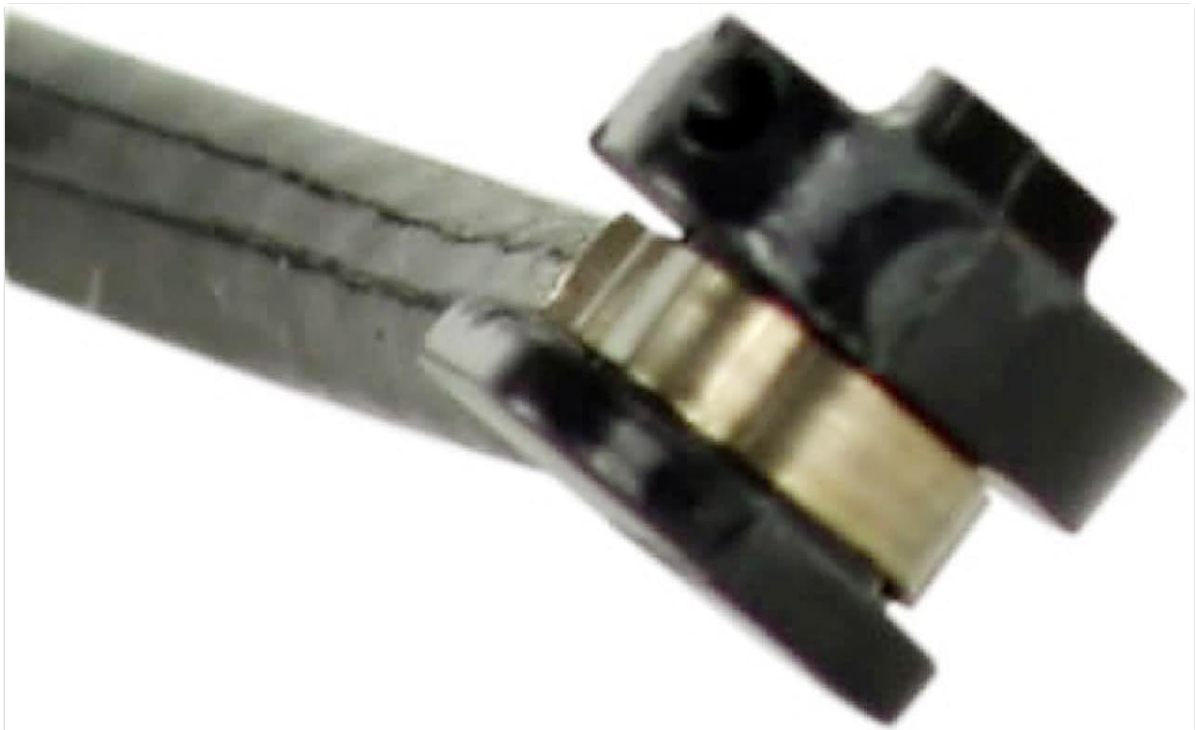
Figure 4.1: Close-up of the sensor's wear tip, which makes contact with the brake rotor.
