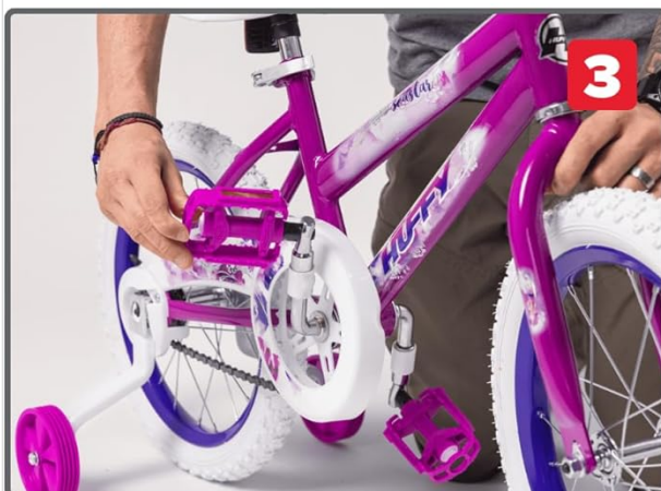
Image: Visual guide for Huffy EZ Build assembly, showing steps for handlebar insertion, pedal folding, and seat adjustment.
