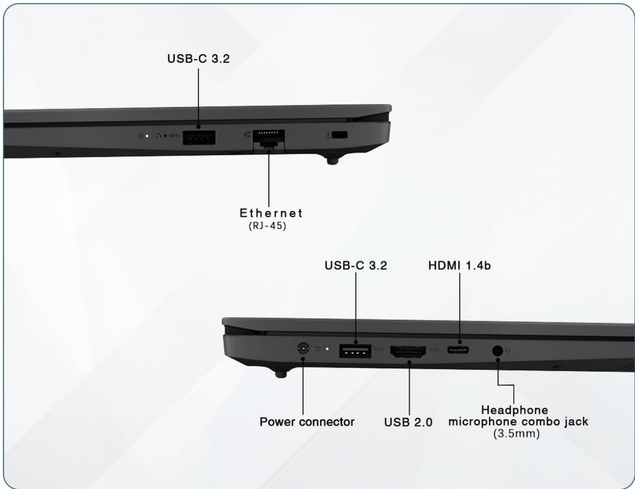
Image: Detailed view of the various connectivity ports on the Lenovo V15 Laptop.
