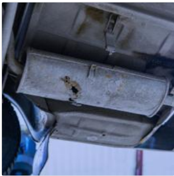
Damaged Muffler: An image showing a rusted and damaged muffler, illustrating a common reason for replacement and a potential source of exhaust issues.
