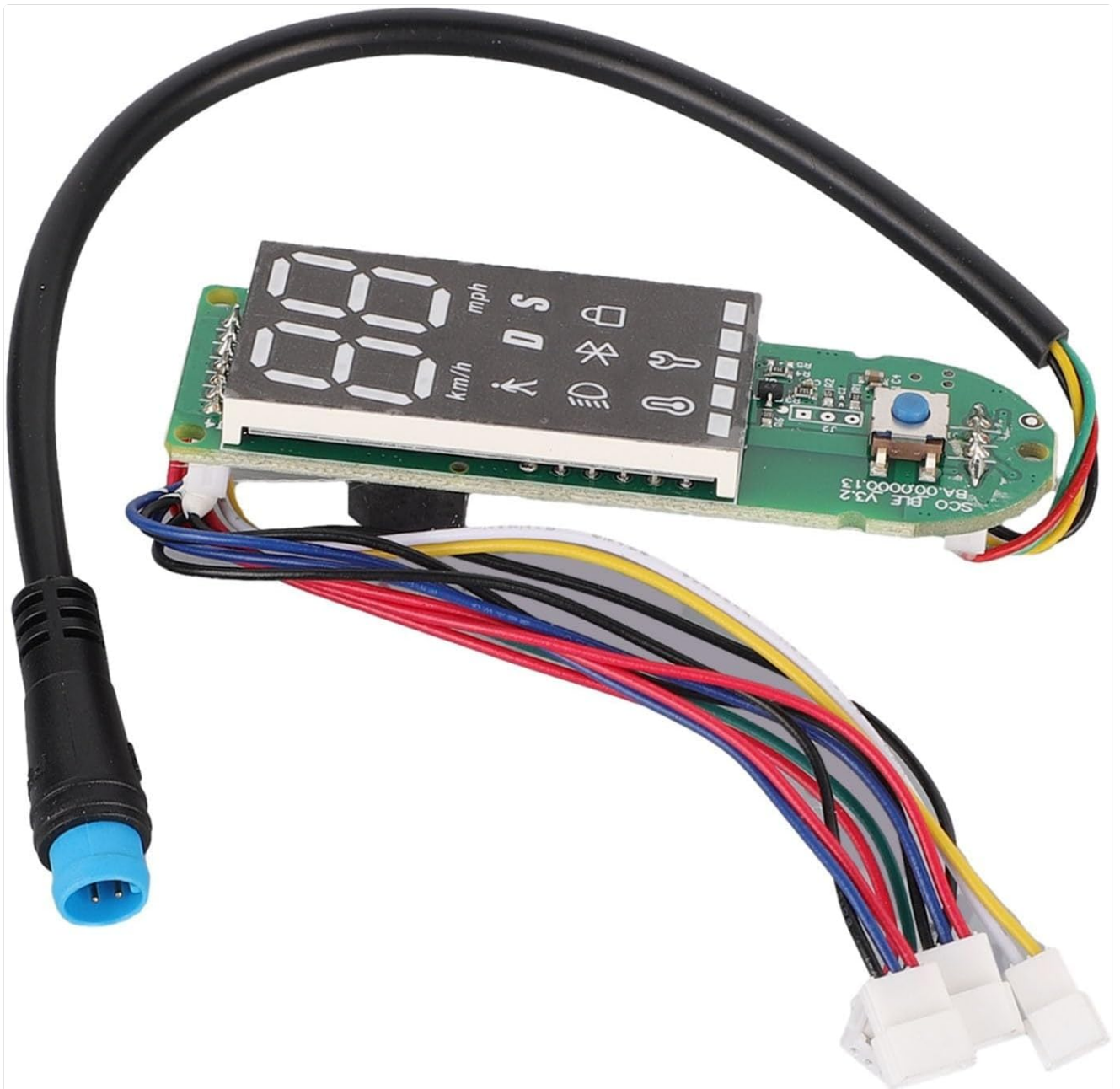
Image: The Bluetooth circuit board with its wiring harness, ready for connection.
