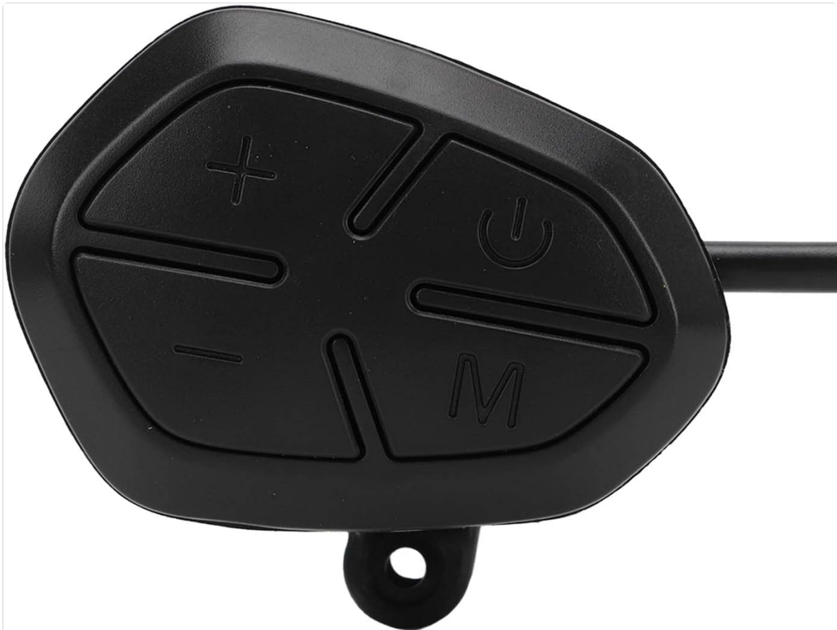
Figure 4.2: The control unit with its five distinct buttons: Power, Mode, Plus (+), Minus (-), and a central button, used for navigating menus and adjusting settings.
