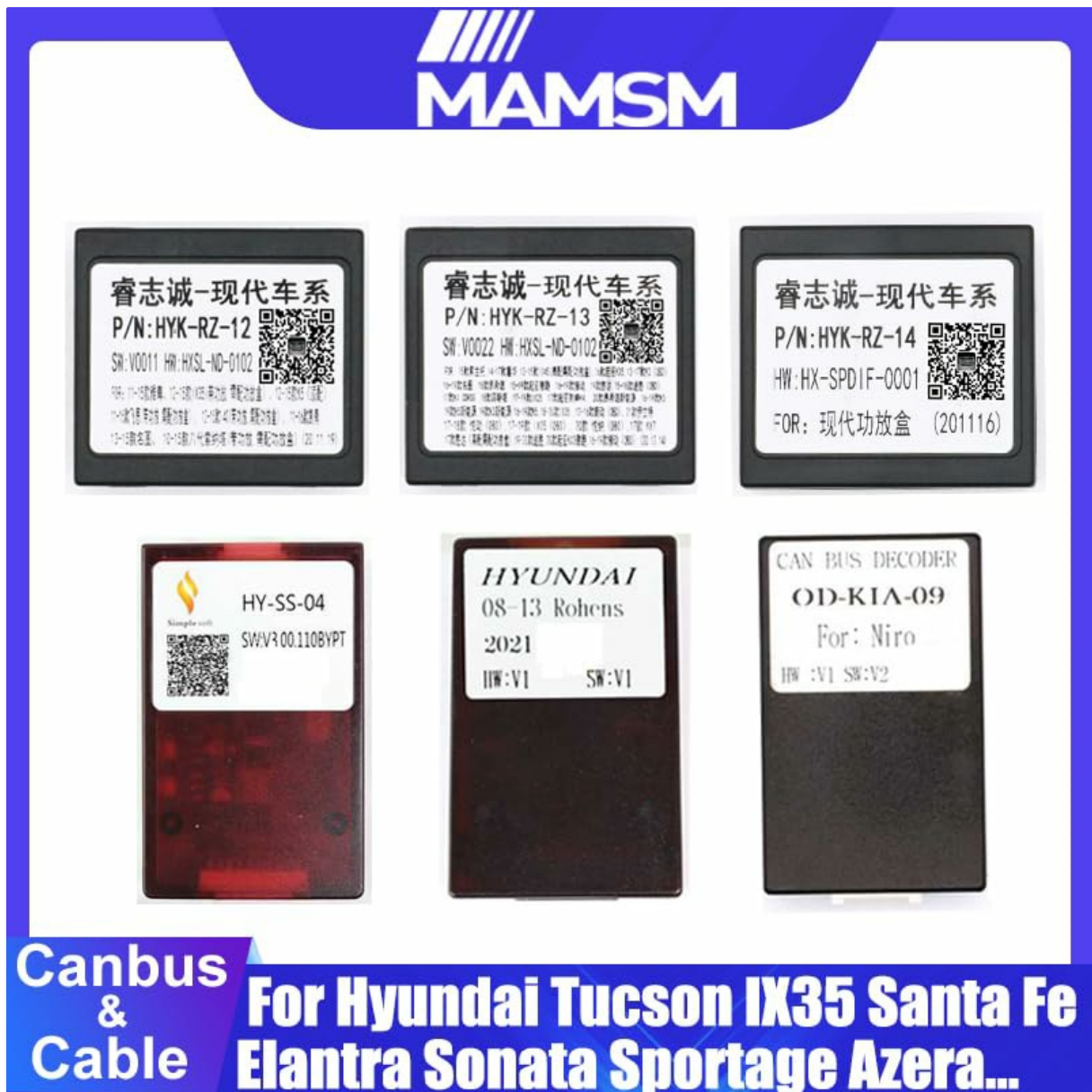
Image 2.2: An assortment of Canbus Decoder Boxes, including models like HYK-RZ-12, HYK-RZ-13, HYK-RZ-14, and HY-SS-04. This illustrates the variety of specific Canbus box models available for different vehicle compatibility requirements.
