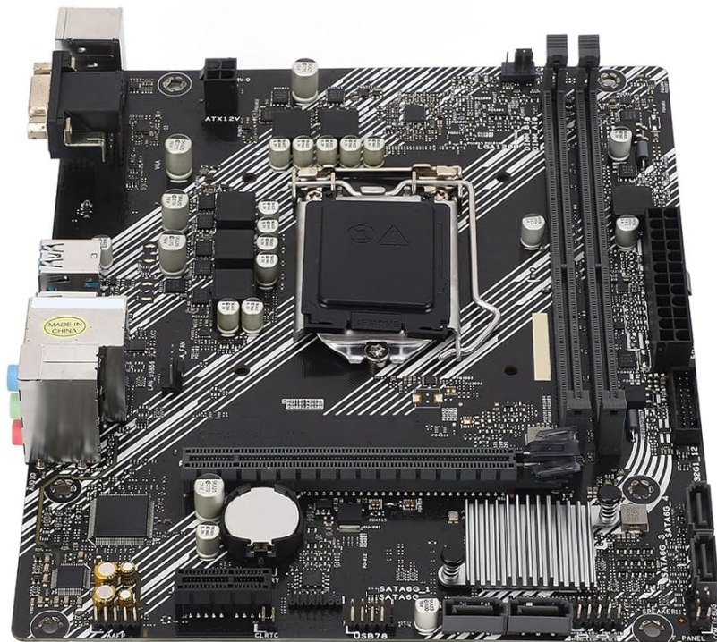
Figure 3.1: The motherboard's VGA interface supports high-definition visuals for connected displays.
